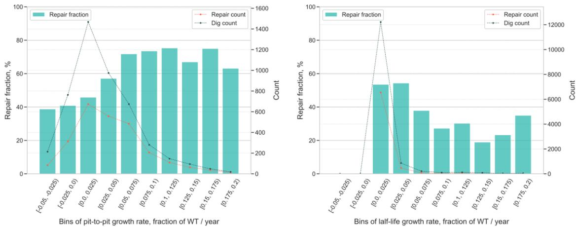
**Figure 7.** Left plot (a): Repair fraction as a function of the pit-to-pit growth. Right plot (b): Repair fraction as a function of the growth based on the half-life calculation.
