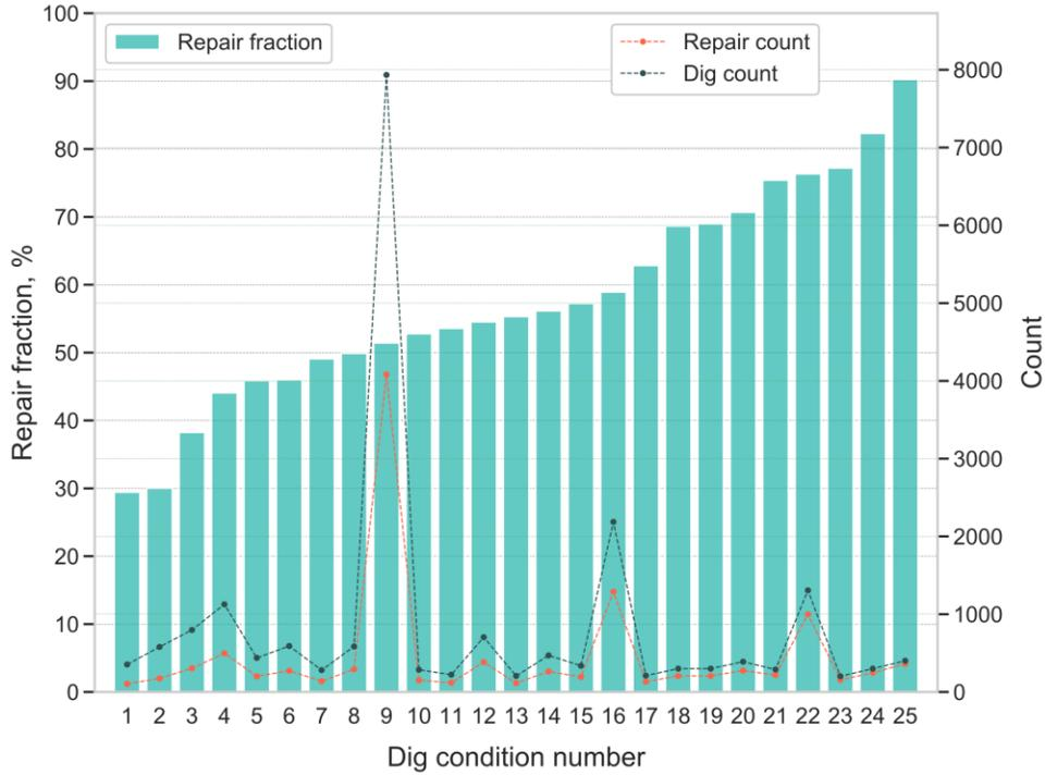
**Figure 3.** Repair fraction plotted across different conditions used in a dig program. The conditions are sorted in the order of increasing repair fraction.
