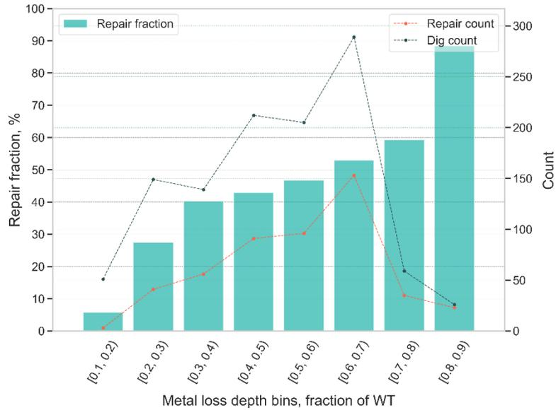
**Figure 4.** Condition 4 repair fraction divided into bins of ILI measured metal loss. The integrated repair fraction ratio is 44.1%
