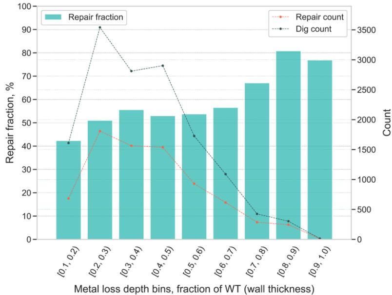
Figure 2. Repair fraction shown as a function of corrosion depth as measured by ILI tools.
